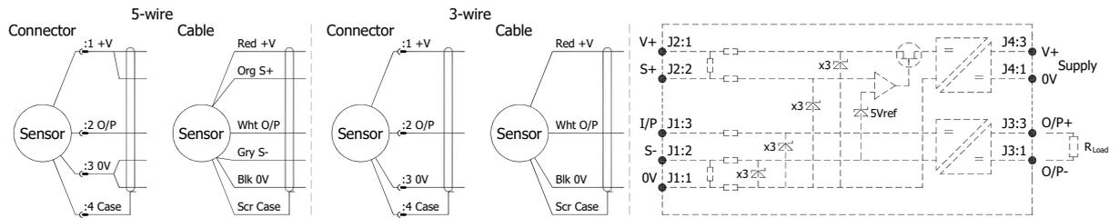
**Putting Into Service:** The sensor must be used with a galvanic isolation barrier designed to supply the sensor with a nominal 5V and to transmit the sensor output to a safe area. The barrier parameters must not exceed:-
