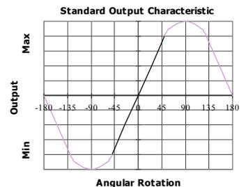
**Output Characteristic:** The sensor has full rotational freedom and two sectors, 180° apart, over which linear response can be achieved. At the mid point of the calibrated range the output signal will be half full scale deflection, and the mounting flanges will be vertical. In the calibrated range the output increases as the sensor is rotated in an anti-clockwise direction viewed from the flange face- see drawing above. The calibrated output is factory set to be between 15° and 160°.
