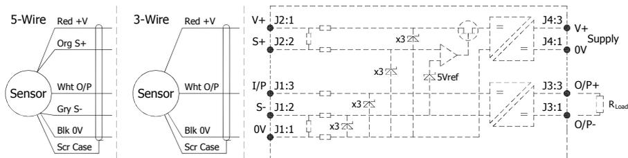
**Putting Into Service:** The sensor must be used with a galvanic isolation barrier designed to supply the sensor with a nominal 5V and to transmit the sensor output to a safe area. The barrier parameters must not exceed:-
