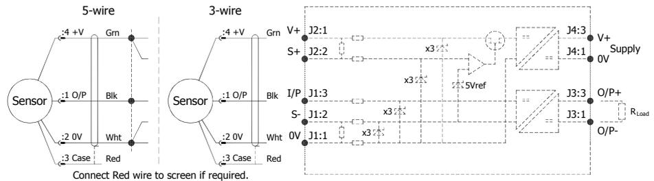
**Putting Into Service:** The sensor must be used with a galvanic isolation barrier designed to supply the sensor with a nominal 5V and to transmit the sensor output to a safe area. The barrier parameters must not exceed:-
